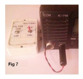
To test both kits, I plugged in the 3.5mm mono jack plugs into their respective filter enclosure sockets and the transceiver mono jack plug to the transceiver phone out socket.
